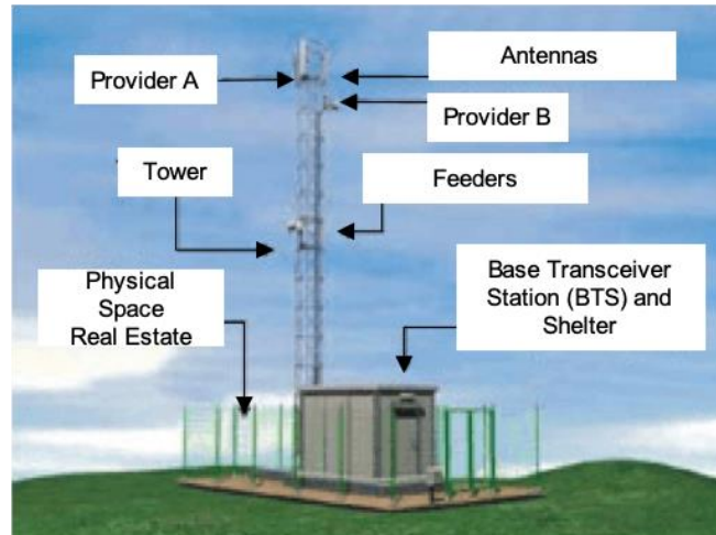
Figure 5-3. Components of a Radio Site
